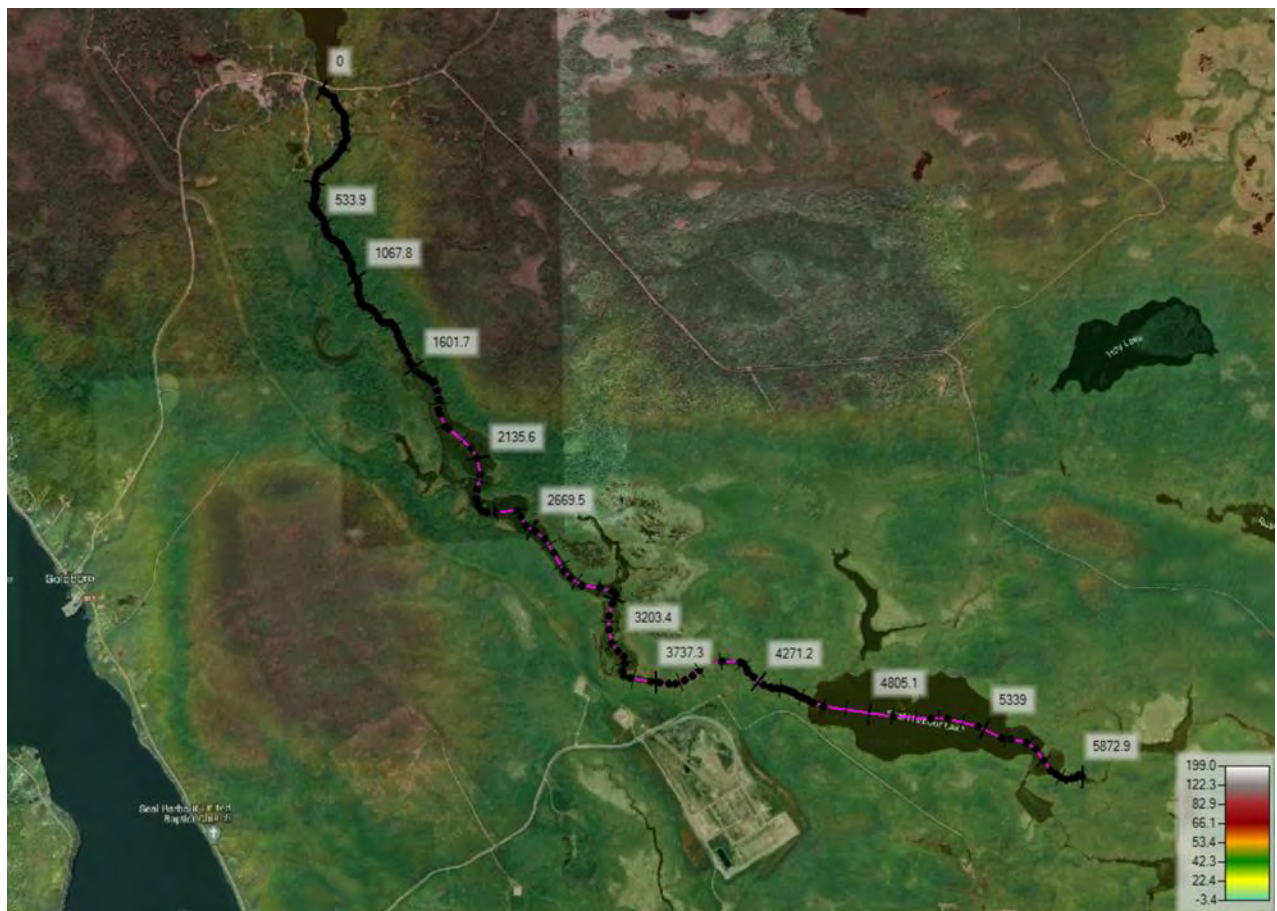
Figure 5 Channel stationing. Aerial imagery and digital elevation model on the background.
